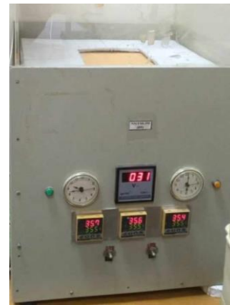
Fig. 16. The thermal resistance test on a 20 cm * 20 cm PET Sample
