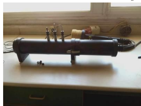
Fig. 18. Two-microphone impedance tube device used in sound absorb and isolation test
