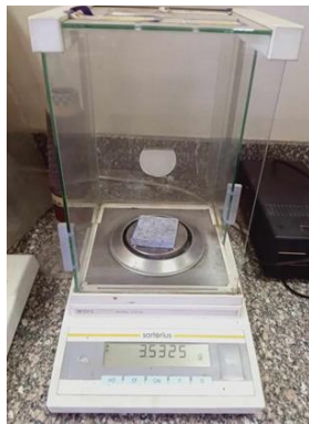
Fig. 13. the process of indicating the weight of a 5 cm * 5 cm PET Sample
