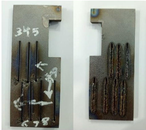
Fig. 4. Samples with defects produced during the first trials of input parameters.
