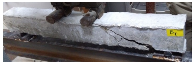
Fig. 9. crack pattern of control beam B_{I0}
