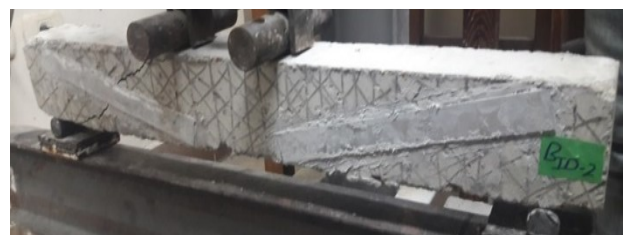
Fig. 12. crack pattern and mode of failure for the beams strengthen using strengthening technique (3).
