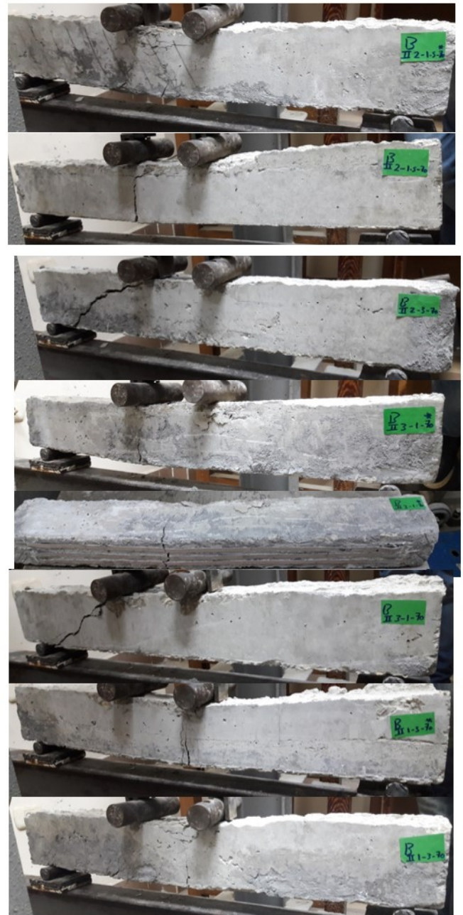
Fig. 15. crack pattern and mode of failure for the beams strengthen using strengthening technique (5).
